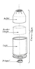
The case is the most expensive element of a completed cartridge and the one which needs to be retained for reloading in order to reduce costs. In principle this can be reloaded
